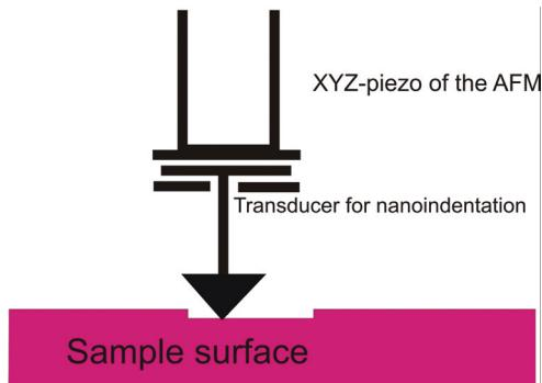
Figure 6: Schematically assembly of the AFM with Nanointender
