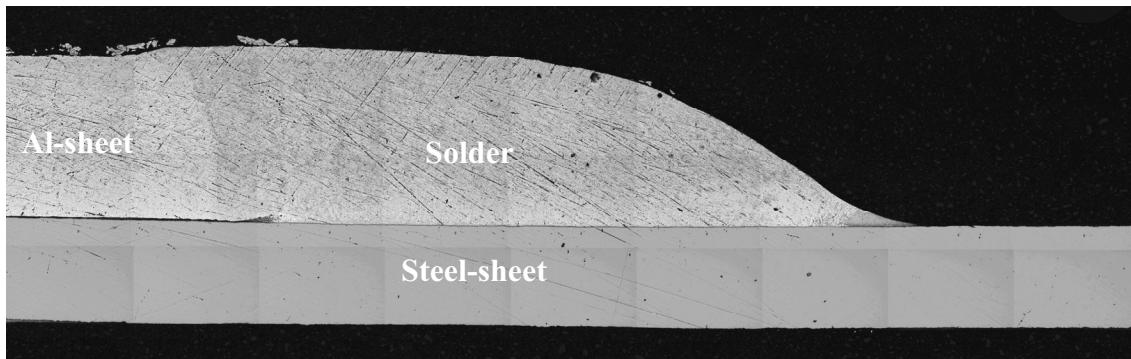
Figure 4: CMT-welding of steel and Aluminum
