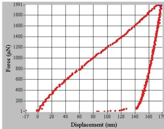
Figure 7: Force-displacement curve as the primary result of the measurement
