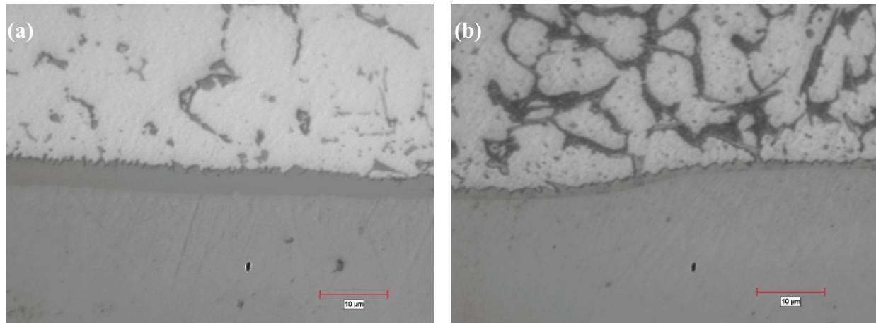
Figure 5: Typical microstructure of CMT-weldings. (a)SSAISiMn, (b)AlSi5. Magn. 1000
