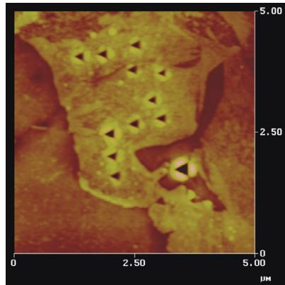
Figure 8: Intends of the measurement with a AFM-Nanoindenter
