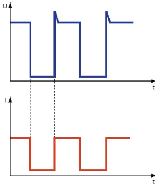
Figure 3: Schematic diagram of current and voltage during the CMT-process
