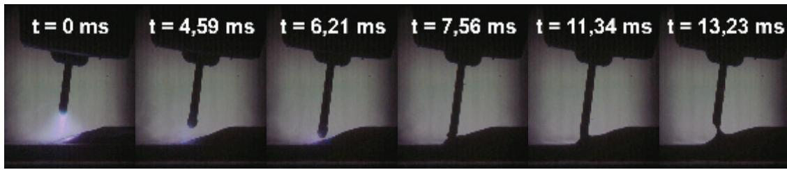
Figure 2: The principle of the CMT-process, where an oscillating wire feeding is performed.
