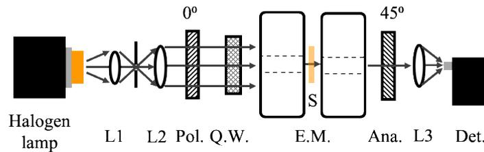
**Fig.1** Magneto-optical multi-channel spectrometer using polarization modulation method
