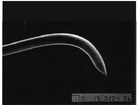
Fig. 2. SEM image of optical fiber probe used in the SNOM/AFM system. The bending angle of the probe is about 80°.
