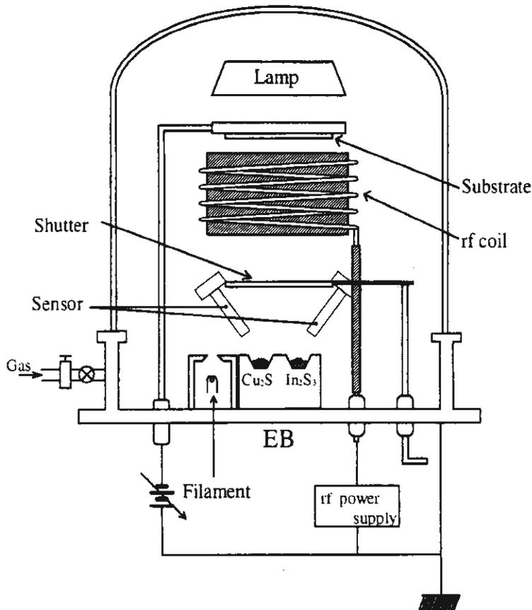
Fig. 1. Schematical illustration of rf ion plating system.
