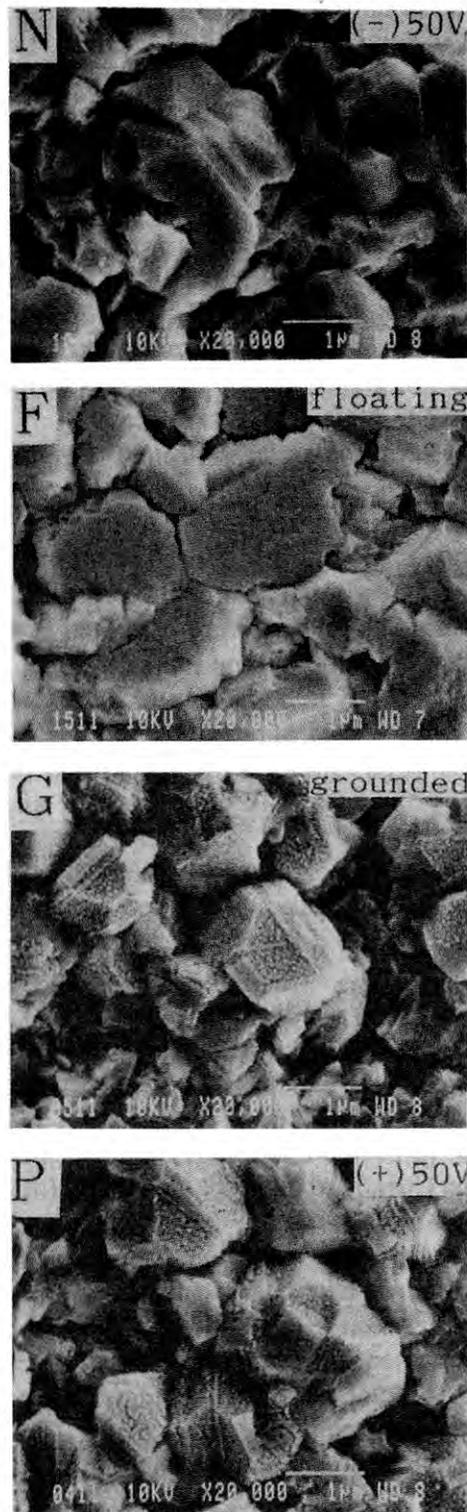
Fig. 5. SEM micrographs showing surface morphology of as-deposited films for various substrate biases: N (– 50 V), F (floating), G (grounded), and P (+ 50 V).
