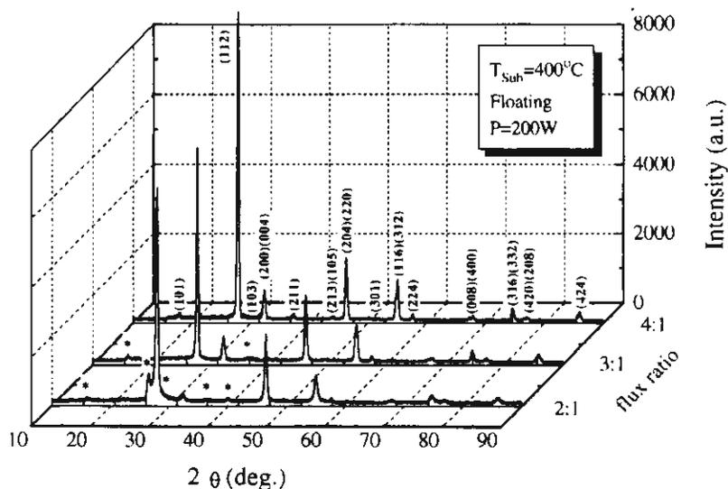
Fig. 2. XRD patterns of films prepared with different flux (i.e.,  $\text{Cu}_2\text{S}/\text{In}_2\text{S}_3$ ) ratios.
