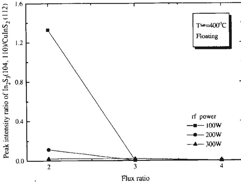
Fig. 3. Plot of XRD peak intensity ratio of  $\text{In}_2\text{S}_3(104, 110)/\text{CuInS}_2(112)$  versus flux ratio for various rf power, after KCN-treatment.
