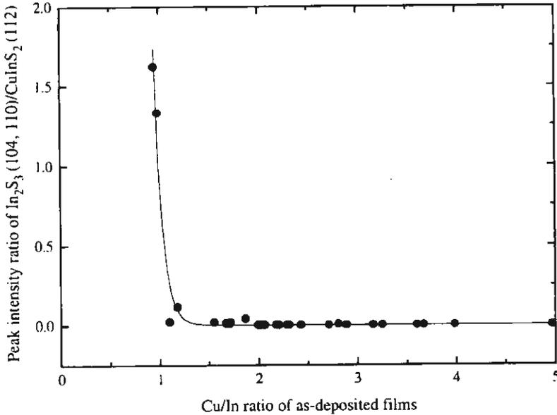
Fig. 4. Plot of XRD peak intensity ratio of  $\text{In}_2\text{S}_3(104, 110)/\text{CuInS}_2(112)$  versus Cu/In ratio of as-deposited films grown at various conditions.
