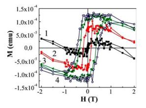
**Fig. 6** (online colour at: www.pss-a.com) Hysteresis loops for the sample with SA nanowhiskers grown at  $520 \,^{\circ}$ C (Fig. 1d) measured at different temperatures: (1) 295 K; (2) 70 K; (3) 30 K; (4) 5 K.
