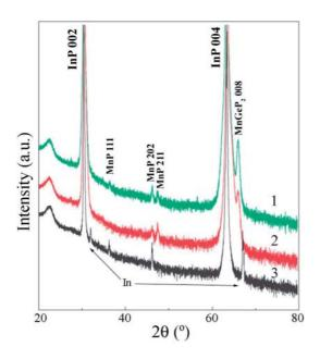
**Fig. 2** X-ray diffraction pattern of samples with SA nanowhiskers grown at 435  $^{\circ}$ C (1) (see Fig. 1a and b); 520  $^{\circ}$ C (2) (see Fig. 1d) and MnP nanowhiskers grown at 545  $^{\circ}$ C (3).
