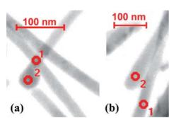
**Fig. 3** Low-resolution STEM images of Ge (a) and MnP (b) nanowhiskers grown at 500 °C (see Fig. 1c). (EDX analysis of the nanowhiskers has been performed for the depicted points).
