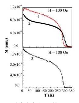
**Fig. 5** (online colour at: www.pss-a.com) Temperature dependence of magnetization measured with an applied field of 100 Oe for (1) the sample with SA nanowhiskers grown at 520 °C (Fig. 1d); (2) MnGeP<sub>2</sub> thin film grown on GaAs(001) substrate with Ge buffer layer [16] and (3) SA nanowhiskers grown at 520 °C peeled off from the InP(001) substrate.
