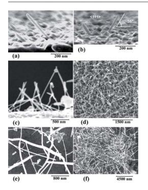
Fig. 1 SEM images of individual (a), (b) and arrays of SA nanowiskers (c), (d) as well as MnP nanowhiskers (e), (f) grown on InP(001) surface. The temperature of the growth: (a), (b) 435 °C; (c) 500 °C; (d) 520 °C; (e), (f) 545 °C.
