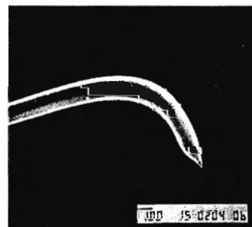
Fig.2 Bent fiber probe used as an AFM cantilever
