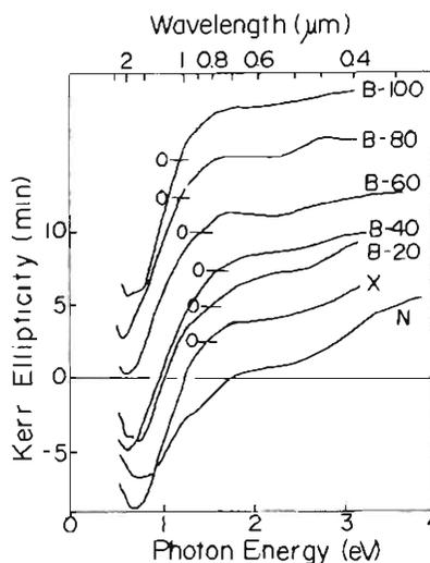
Fig. 2. Kerr ellipticity spectra of amorphous Gd-Co films prepared under various sputtering conditions. About symbols, N, B, and X, see the text. Zero-level of each curve is shifted by arbitrary amount for the sake of clarity.
