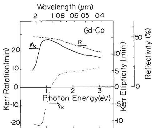
Fig. 1. Kerr rotation  $\phi_K$ , Kerr ellipticity  $\eta_K$ , and reflectivity  $R$  of Gd-Co film measured through substrate glass. Solid curve:  $\phi_K$ , dotted curve:  $\eta_K$ , and dashed curve:  $R$ .
