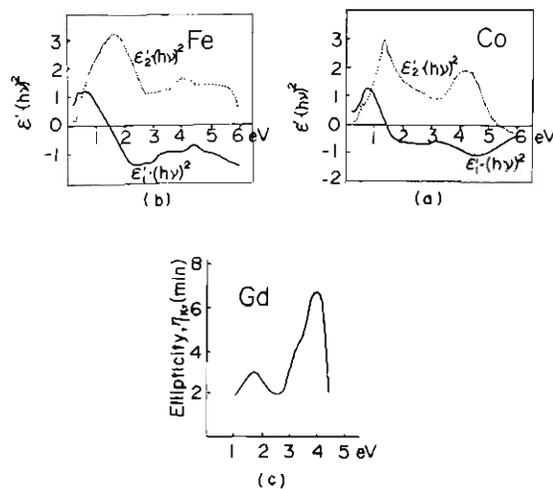
Fig. 4. Magneto-optical spectra of (a) Co; (b) Fe; (after Krinchik and Artemjev [8]), and (c) Gd; (after Erskine and Stern [9]).
