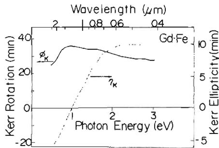
Fig. 3. Kerr rotation spectrum and Kerr ellipticity spectrum of a Gd-Fe film. Solid curve:  $\phi_K$  and dotted curve:  $\eta_K$ .
