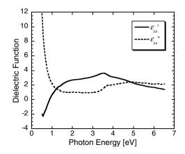
Fig. 1. Real and imaginary part of dielectric functions of BSCCO single crystals.
