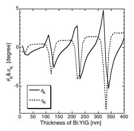
Fig. 3. Thickness dependence of  $\theta_{\rm K}$  and  $\eta_{\rm K}$  for Bi:YIG/BSCCO/STO structures.
