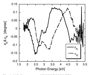
Fig. 6. MO Kerr spectra of Bi:YIG/BSCCO/STO structures.
