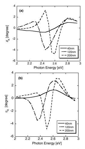
Fig. 2. Calculation of: (a) Kerr rotation  $\theta_{\rm K}$  and (b) Kerr ellipticity  $\eta_{\rm K}$  for Bi:YIG/BSCCO/STO structures.
