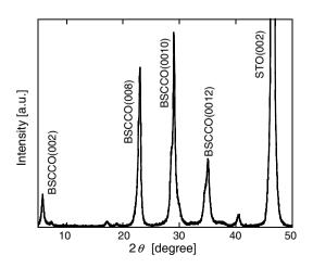
Fig. 4. XRD patterns of Bi:YIG/BSCCO/STO structures.
