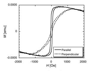
Fig. 5. M-H loops of Bi:YIG/BSCCO/STO structures.
