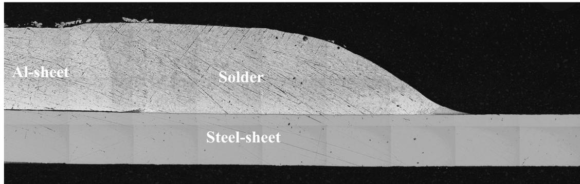
Figure 4: CMT-welding of steel and Aluminum
