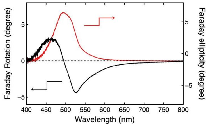
**Fig.2** Faraday rotation and ellipticity spectra of Bi:NIG thin film on GGG substrate.
