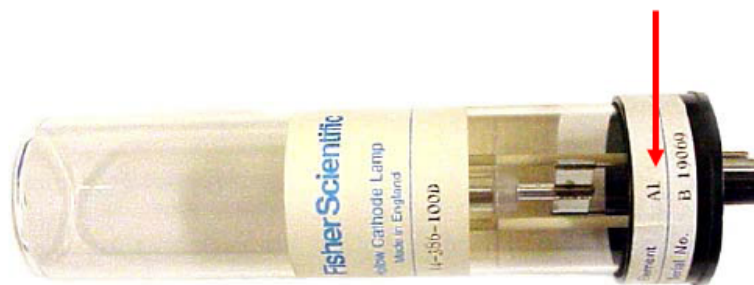
A hollow cathode lamp for Aluminum (Al)
