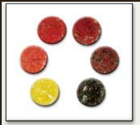
Mixed crystals of yellow cadmium sulfide CdS and black cadmium selenide CdSe, showing the intermediate-band-gap colors
